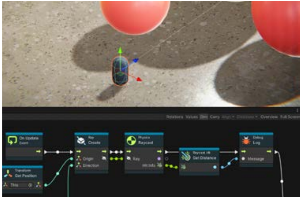
Our capsule has a ray cast in front that outputs the distance to the nearest collision hit. It's drawn on the screen using drawLine.
