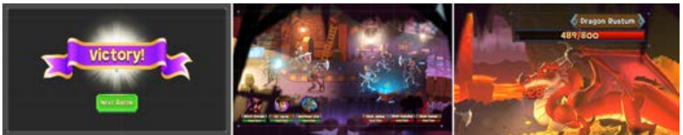
Examples of UI rendering modes, from left to right: Screen Space – Overlay, for screens that absolutely overlay everything else. Screen Space – Camera, is useful for context-specific UI, and World Space UI Canvases creates elements that need to appear in the game world space.
