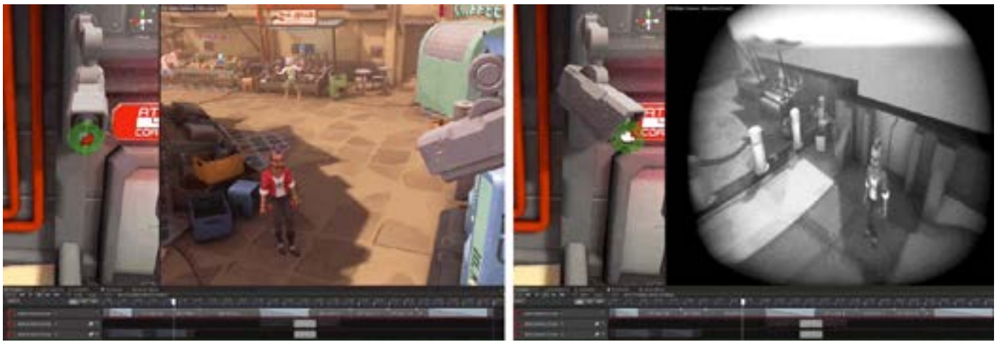
In the example above, a local post-processing volume gives the impression of looking through the lens of an old security camera.
