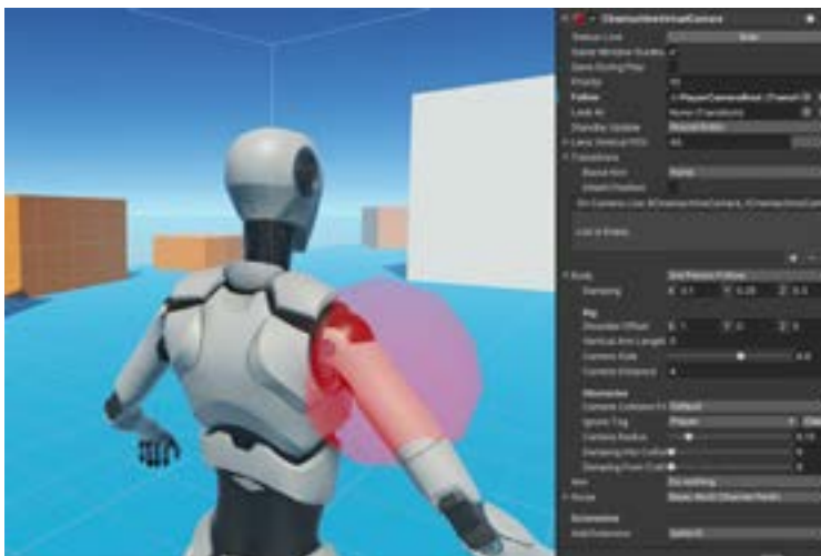
The Third Person asset pack uses a Cinemachine camera with settings designed for a Third Person Follow, such as options to avoid camera obstacles.
